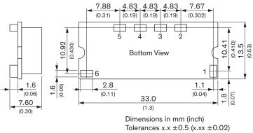
Tolerances x.x  $\pm 0.5$  (x.xx  $\pm 0.02$ ) Tolerances x.xx  $\pm 0.25$  (x.xxx  $\pm 0.01$ ) Pin dimension tolerance  $\pm 0.1$  ( $\pm 0.004$ )
